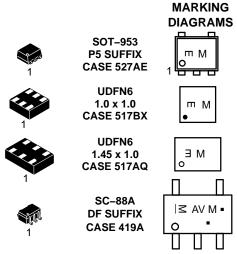
E = Specific Device Code (E with 90 degree clockwise rotation)
