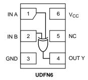
Figure 1. Pinouts (Top View)
