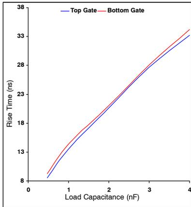
**Figure 6. Driver Rise Time vs. Load Capacitance**
