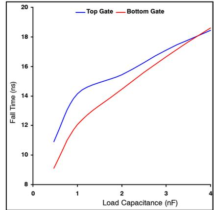
**Figure 5. Driver Fall Time vs. Load Capacitance**
