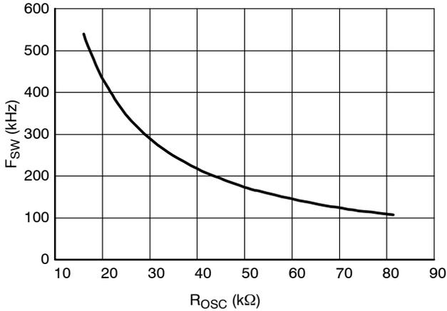
Figure 23. Frequency vs. R<sub>OSC</sub>
