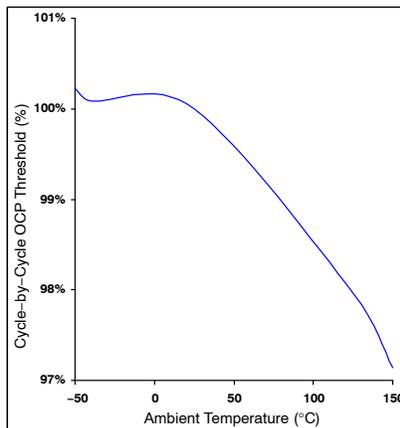
**Figure 10. Cycle-by-Cycle Overcurrent Protection Threshold vs. Temperature**
