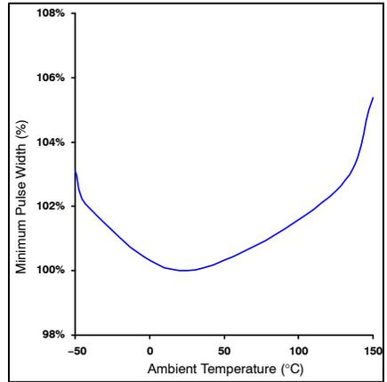
**Figure 14. GH Minimum Pulse Width vs. Temperature**
