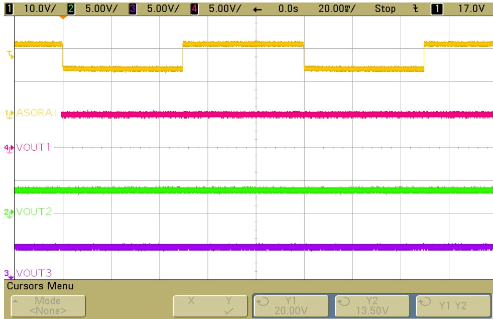
Figure 36. Output Response to OVS – VBAT-MON Left Open
