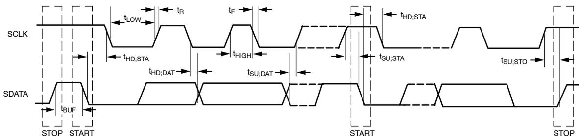
**Figure 3. I<sup>2</sup>C Timing Diagram**
