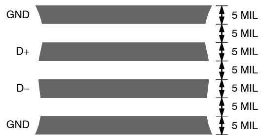
Figure 22. Typical Arrangement of Signal Tracks
