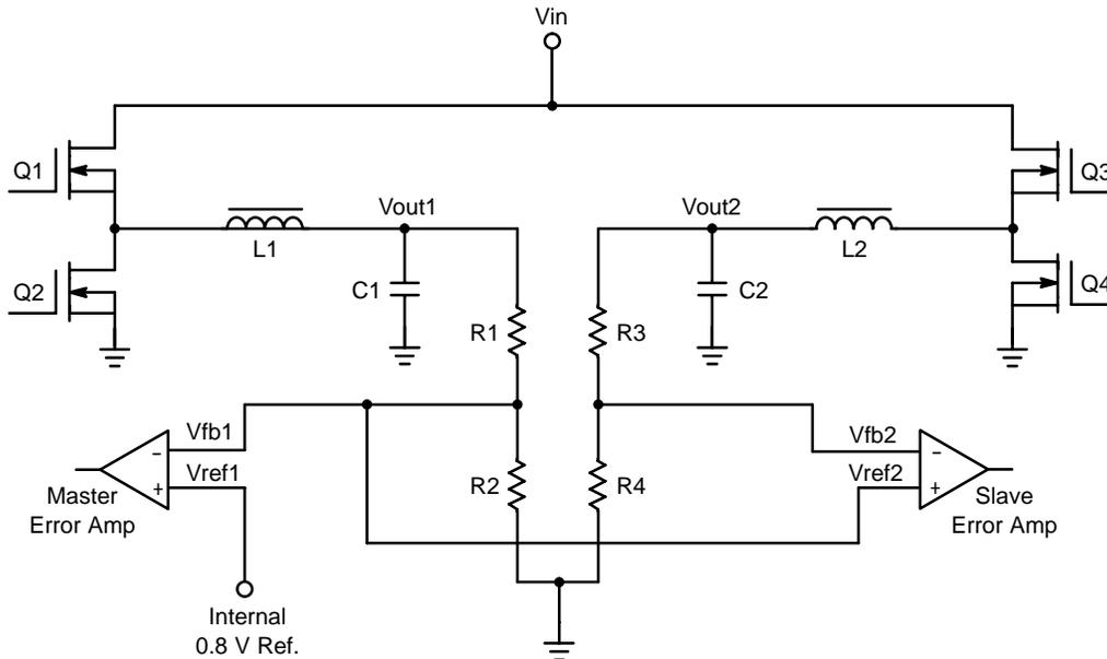
Figure 15. Dual Output Configuration
