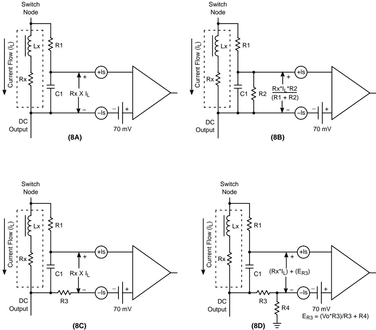
**Figure 8. Inductor Current Sensing – Circuit Configurations**
