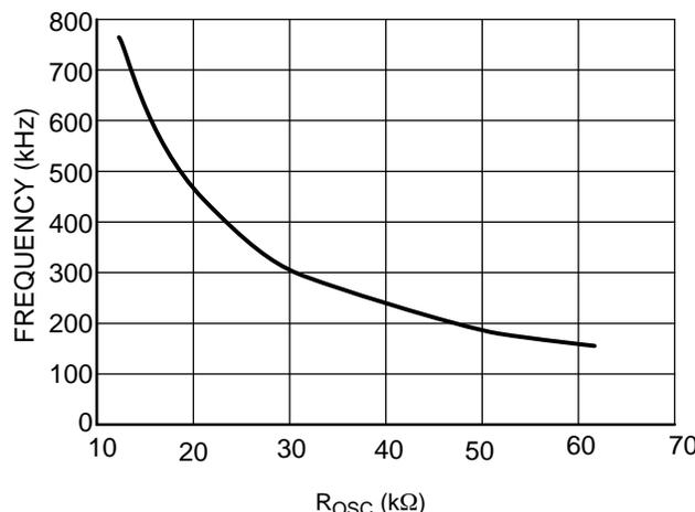
**Figure 10. Switching Frequency vs. R<sub>OSC</sub>**
