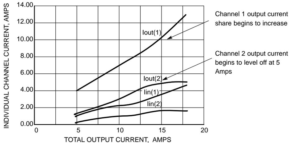
**Figure 7. 70%/30% Current Sharing with Channel 2 Current Limiting**
