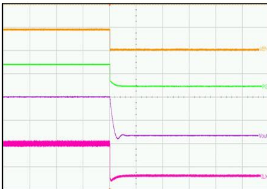
(VIN = 5 V, VOUT = 1.8 V, IOUT = 3 A) Upper Trace: Enable Pin Voltage, 5 V / div Second Trace: Power Good Pin Voltage, 5 V / div Third Trace: Output Voltage, 2 V / div Lower Trace: Inductor Current, 2 A / div Time = 200 \mu s / div
