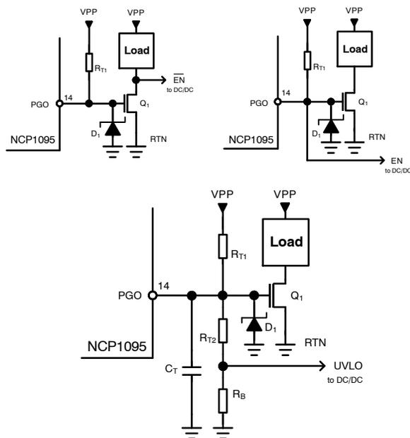
**Figure 5. PGO Interfacing**
