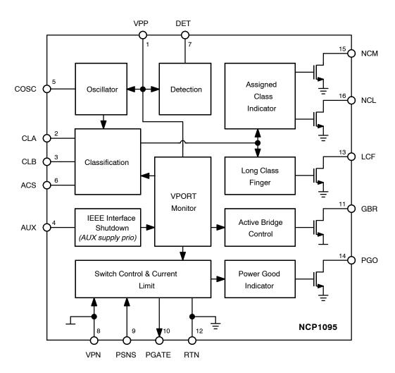
Figure 2. NCP1095 Block Diagram
