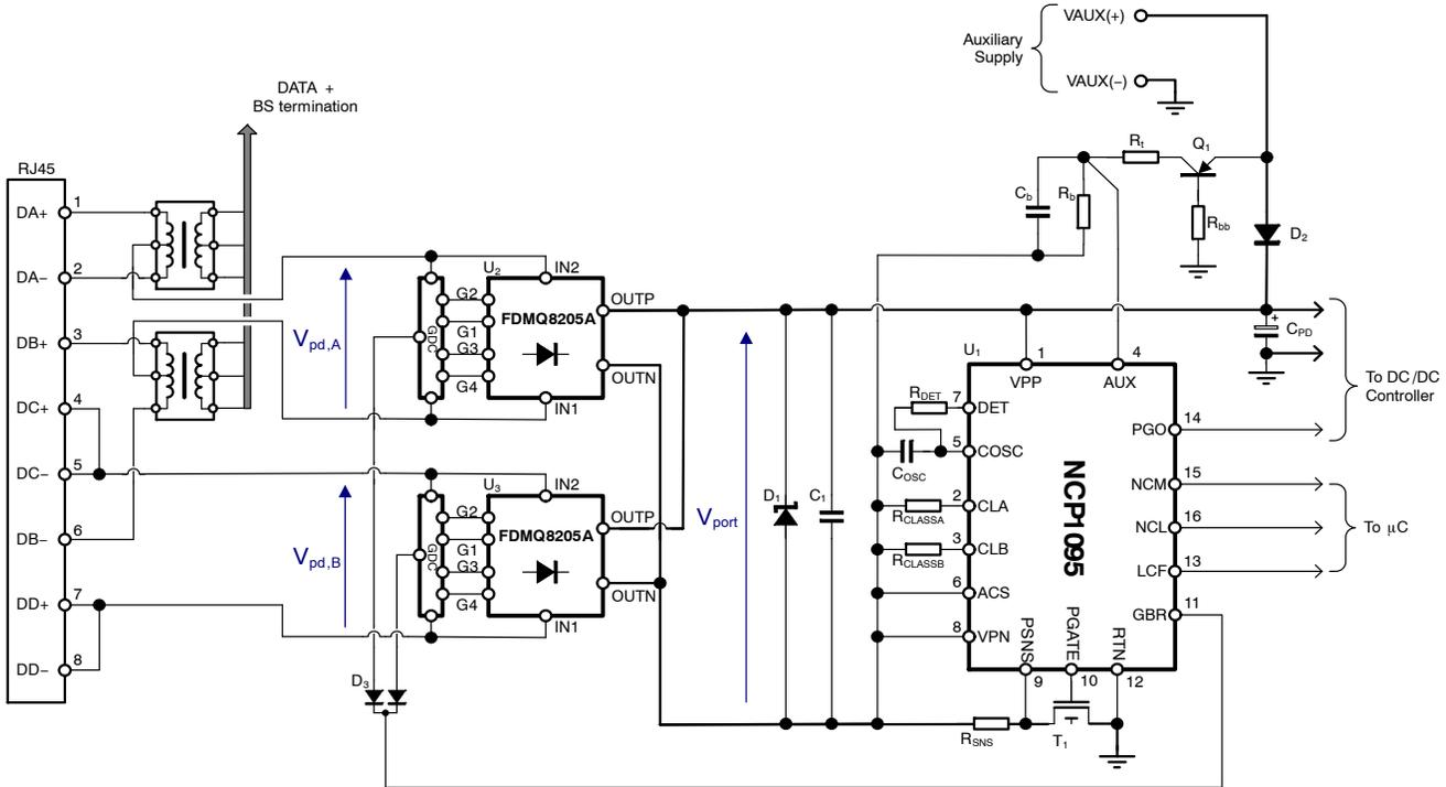
Figure 9. General Application Schematic with Auxiliary Supply
