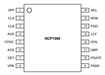
Figure 1. Pin-out NCP1095 in 16-pin TSSOP (Top View)
