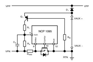
Figure 8. AUX Pin Interfacing
