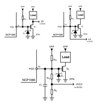
Figure 5. PGO Interfacing
