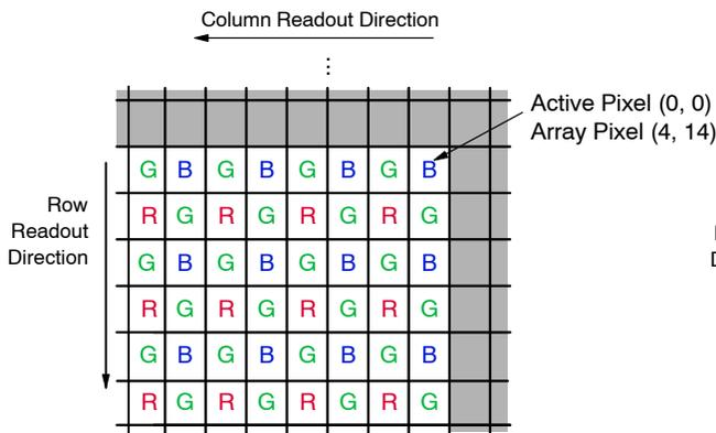
**Figure 5. Pixel Color Pattern Detail (Top Right Corner)**
