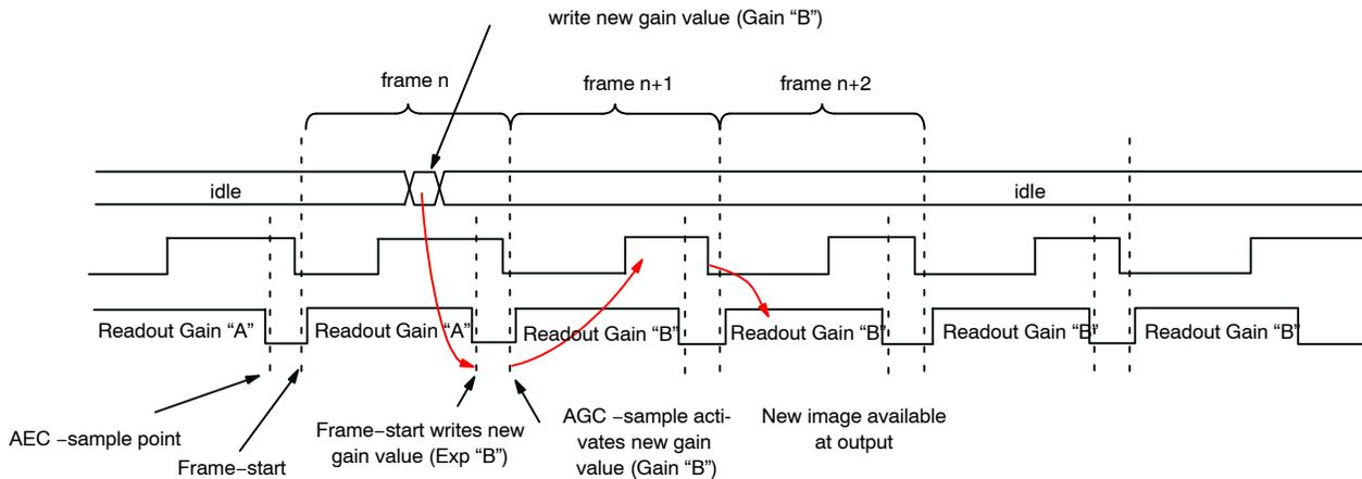
Figure 26. Latency of Gain Register(s) in Master Mode
