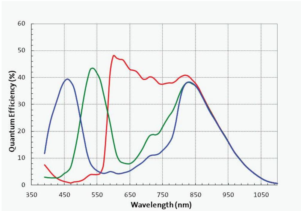
**Figure 47. Typical Quantum Efficiency – RGB Bayer**
