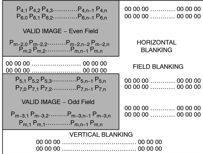
**Figure 34. Spatial Illustration of Interlaced Image Readout**
