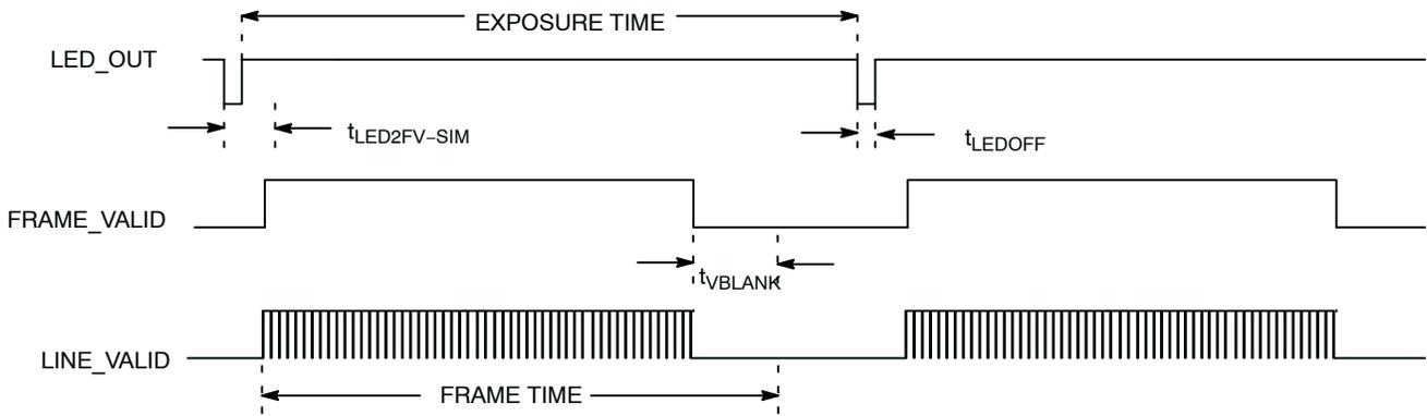
**Figure 15. Simultaneous Master Mode Synchronization Waveforms #2**
