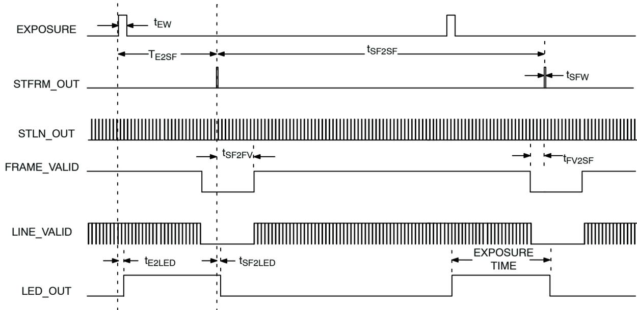
Figure 19. Exposure and Readout Timing (Simultaneous Mode)
