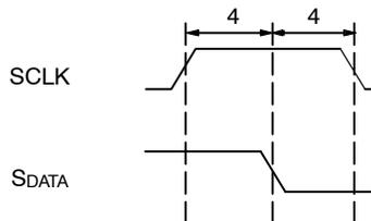
**Figure 41. Serial Host Interface Start Condition Timing**
