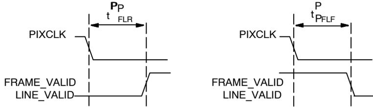
**Figure 39. Propagation Delays for FRAME\_VALID and LINE\_VALID Signals**
