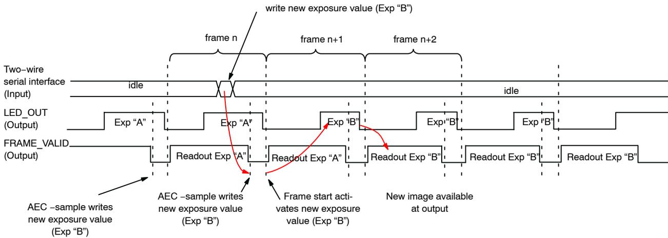
Figure 22. Latency of Exposure Register in Master Mode
