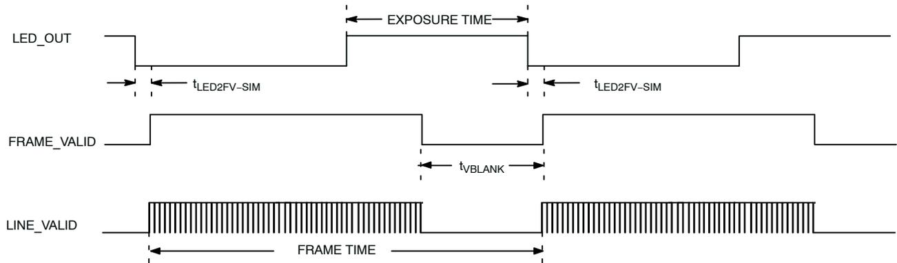
**Figure 14. Simultaneous Master Mode Synchronization Waveforms #1**
