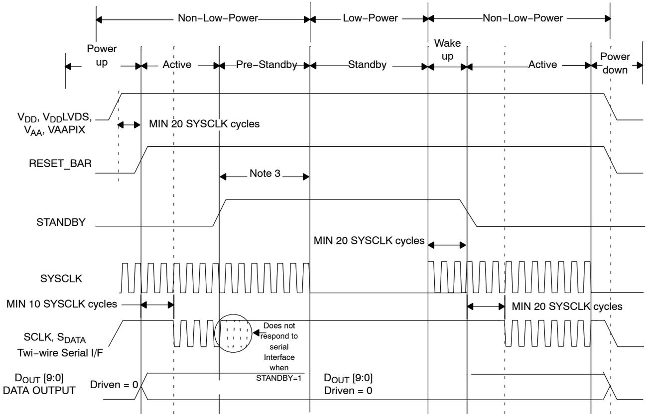
**Figure 50. Power-up, Reset, Clock, and Standby Sequence**
