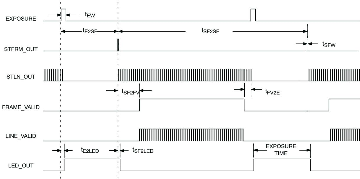
**Figure 20. Exposure and Readout Timing (Sequential Mode)**
