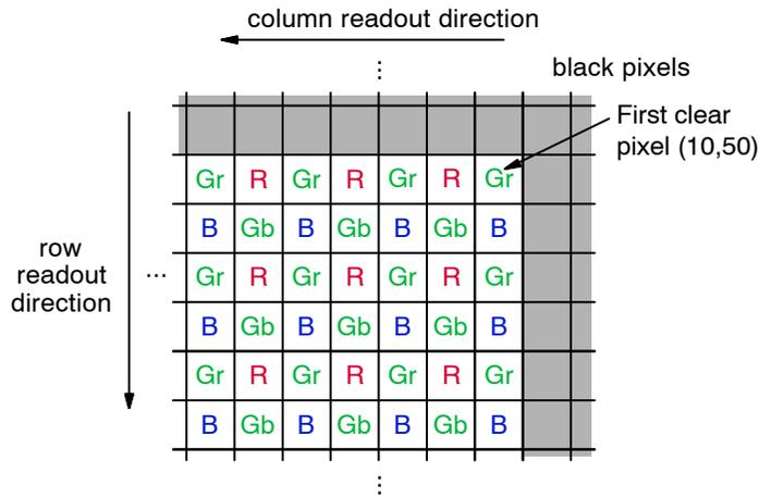
**Figure 5. Pixel Color Pattern Detail (Top Right Corner)**
