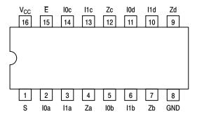
Figure 1. 16-Lead Pinout (Top View)
