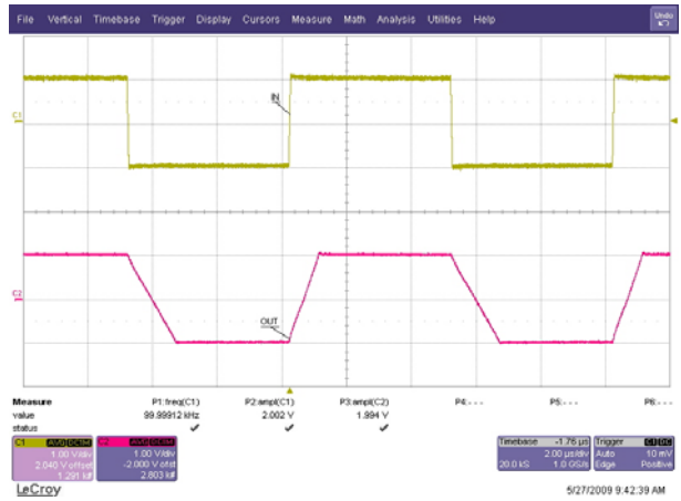
Figure 10. Non-Inverting Large Signal Step Response
