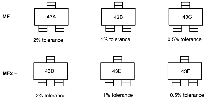
Figure 2. Top Mark (per package)
