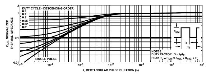
FIGURE 3. NORMALIZED MAXIMUM TRANSIENT THERMAL IMPEDANCE
