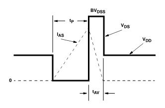
FIGURE 15. UNCLAMPED ENERGY WAVEFORMS
