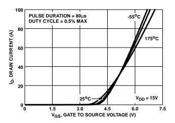
FIGURE 8. TRANSFER CHARACTERISTICS
