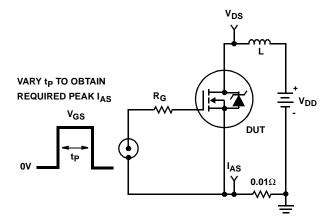
FIGURE 14. UNCLAMPED ENERGY TEST CIRCUIT
