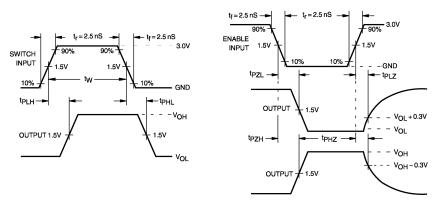
FIGURE 2. AC Waveforms
