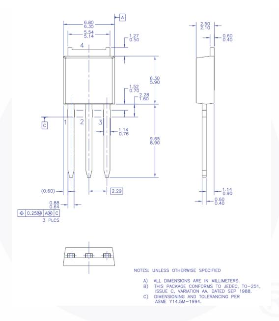
Figure 16. TO-251 (I-PAK), Molded, 3-Lead, Option AA
