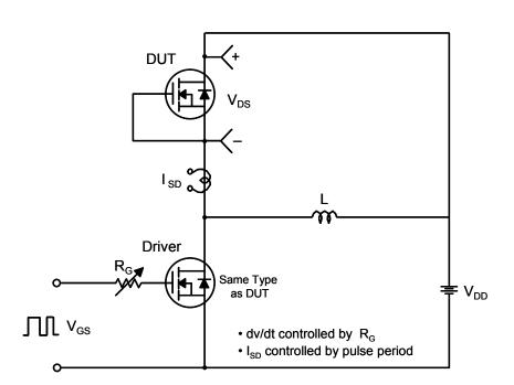
Figure 15. Peak Diode Recovery dv/dt Test Circuit & Waveforms
