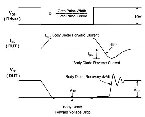
Figure 15. Peak Diode Recovery dv/dt Test Circuit & Waveforms
