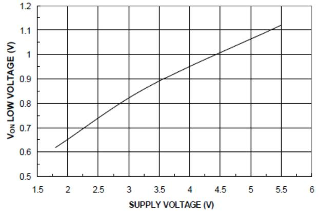
Figure 7. V<sub>ON</sub> Low Voltage vs. Input Voltage
