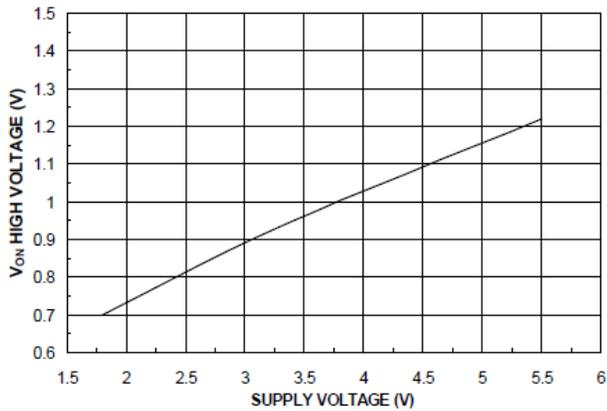
Figure 6. V<sub>ON</sub> High Voltage vs. Input Voltage
