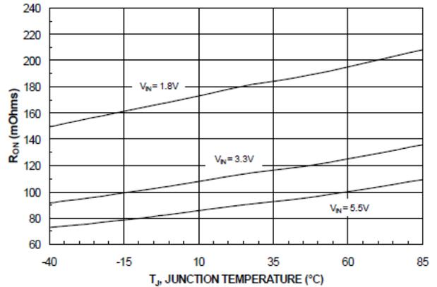
Figure 9. R<sub>ON</sub> vs. Temperature
