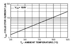
Figure 7. Collector Cut-Off Current vs. Ambient Temperature
