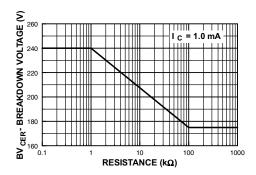
Figure 8. Collector-Emitter Breakdown Voltage with Resistance Between Emitter-Base
