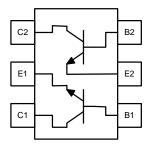
Figure 2. Internal Connection
