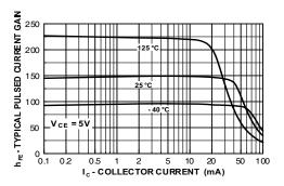
Figure 3. Typical Pulsed Current Gain vs. Collector Current
