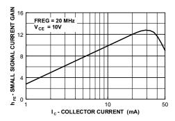
Figure 10. Small Signal Current Gain vs. Collector Current
