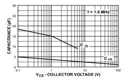
Figure 9. Input and Output Capacitance vs. Reverse Voltage
