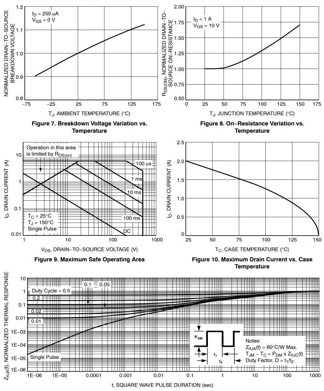
Figure 11. Transient Thermal Response
