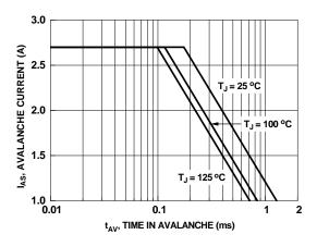
Figure 9. Unclamped Inductive Switching Capability
