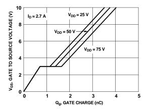
Figure 7. Gate Charge Characteristics
