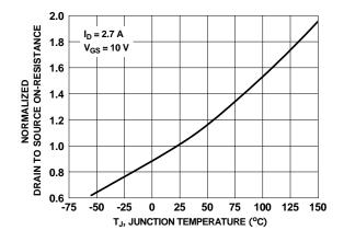
Figure 3. Normalized On-Resistance vs Junction Temperature
