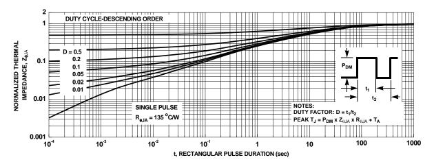
Figure 14. Junction-to-Ambient Transient Thermal Response Curve
