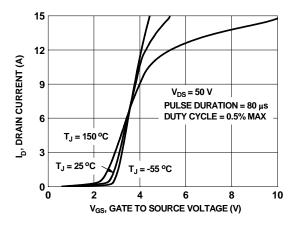
Figure 5. Transfer Characteristics
