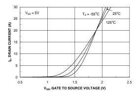
Figure 5. Transfer Characteristics.
