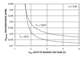
Figure 4. On-Resistance Variation with Gate-to-Source Voltage.
