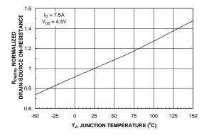
Figure 3. On-Resistance Variation with Temperature.
