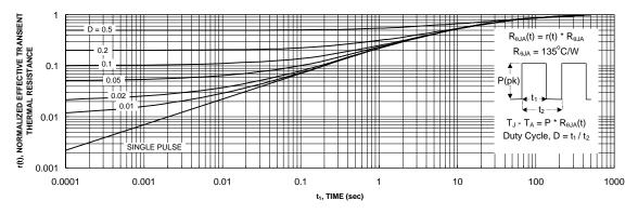
Figure 11. Transient Thermal Response Curve.
