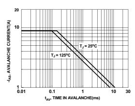
Figure 9. Unclamped Inductive Switching Capability
