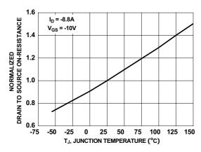
Figure 3. Normalized On-Resistance vs Junction Temperature
