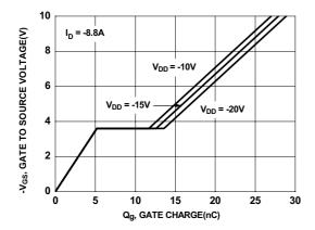
Figure 7. Gate Charge Characteristics
