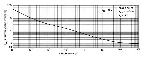
Figure 13. Single Pulse Maximum Power Dissipation
