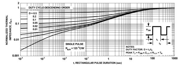
Figure 14. Transient Thermal Response Curve
