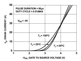
Figure 5. Transfer Characteristics
