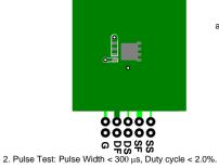
a. 45 °C/W when mounted on a 1 in<sup>2</sup> pad of 2 oz copper.
