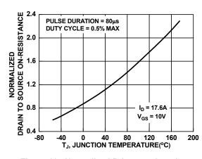
Figure 12. Normalized Rdson vs Junction Temperature
