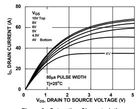
Figure 9. Saturation Characteristics
