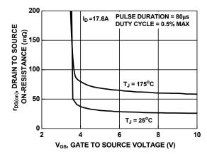
Figure 11. Rdson vs Gate Voltage
