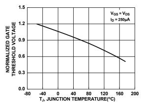
Figure 13. Normalized Gate Threshold Voltage vs
