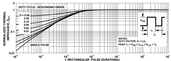
Figure 3. Normalized Maximum Transient Thermal Impedance
