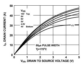
Figure 10. Saturation Characteristics
