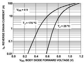
Figure 8. Forward Diode Characteristics
