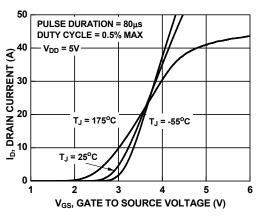
Figure 7. Transfer Characteristics
