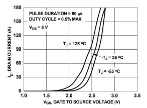
Figure 5. Transfer Characteristics
