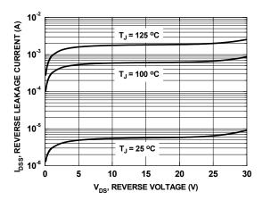
Figure 15. SyncFET<sup>TM</sup> Body Diode Reverse Leakage vs. Drain-Source Voltage
