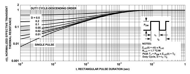
Figure 13. Junction-to-Case Transient Thermal Response Curve
