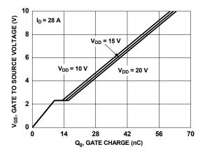
Figure 7. Gate Charge Characteristics
