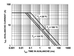
Figure 9. Unclamped Inductive Switching Capability
