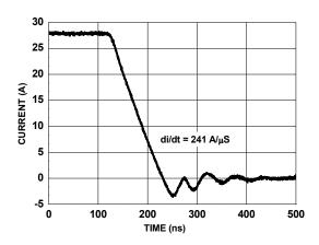
Figure 14. FDMS2D4N03S SyncFET<sup>TM</sup> Body Diode Reverse Recovery Characteristic
