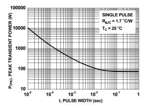
Figure 12. Single Pulse Maximum Power Dissipation
