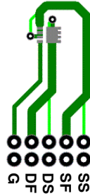
b) 125°C/W when mounted on a minimum pad of 2 oz copper
