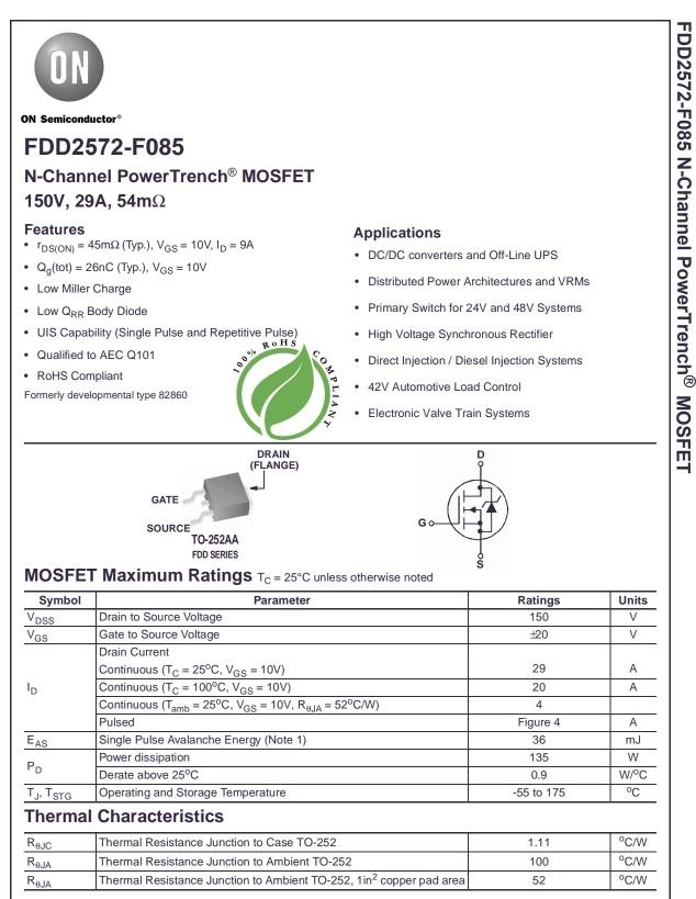
This product has been designed to meet the extreme test conditions and environment demanded by the automotive industry. For a copy of the requirements, see AEC Q101 at: http://www.aecouncil.com/
