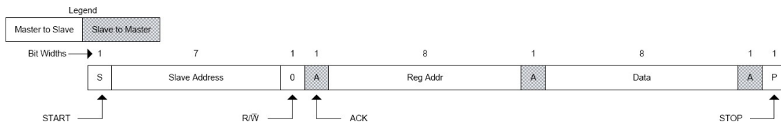
Figure 39. Single Register Write Transaction
