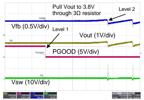
Figure 23. Over-Voltage Protection Level 1 and Level 2
