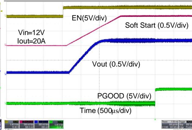
Figure 13. Startup Waveforms with 20 A Load Current
