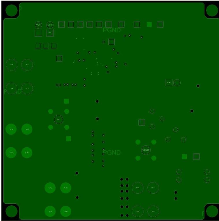
Figure 26. Evaluation Board Inner Layers 2,3, and 4 Copper
