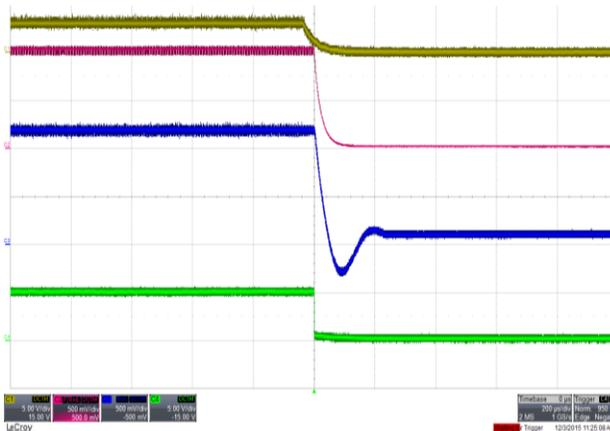
Figure 14. Shutdown Waveforms with 20 A Load Current
