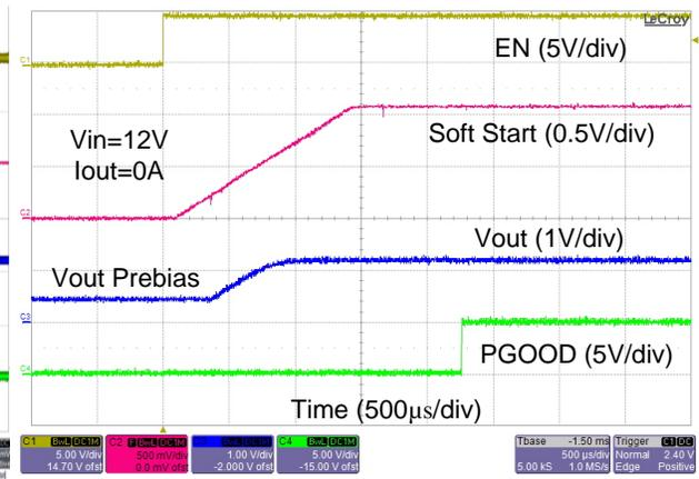
Figure 15. Startup Waveforms with Prebias Voltage on Output
