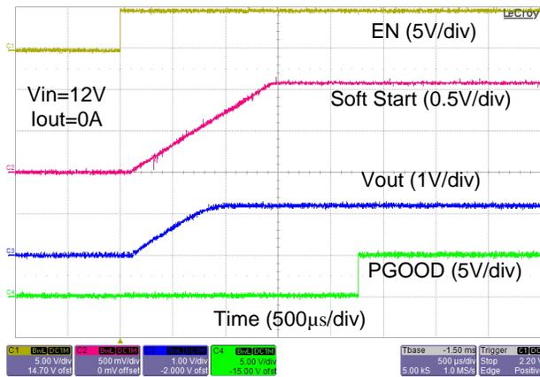
Figure 12. Startup Waveforms with 0 A Load Current
