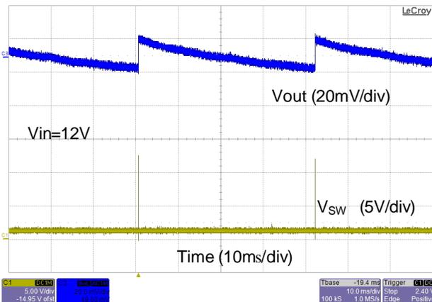
Figure 16. Static Load Ripple at No Load
