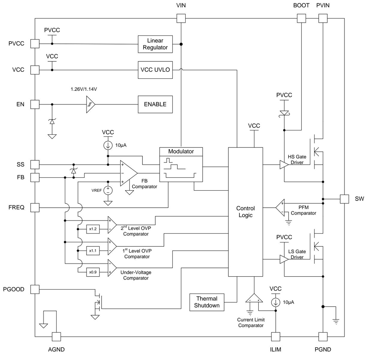
Figure 3. Block Diagram
