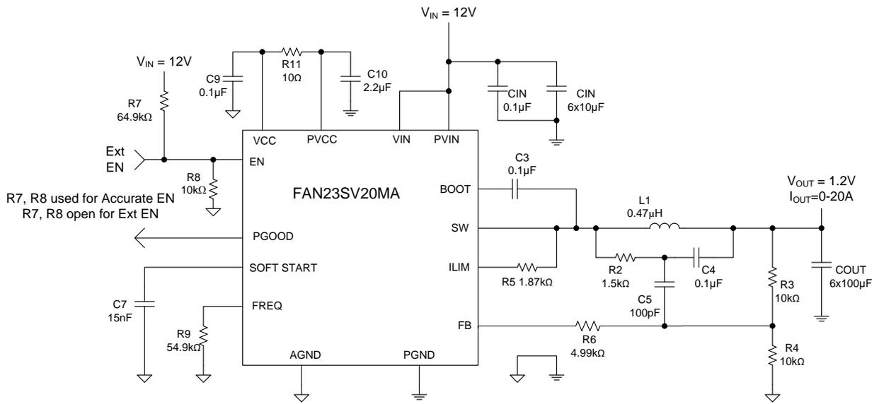
Figure 1. Typical Application with  $V_{IN} = 12V$
