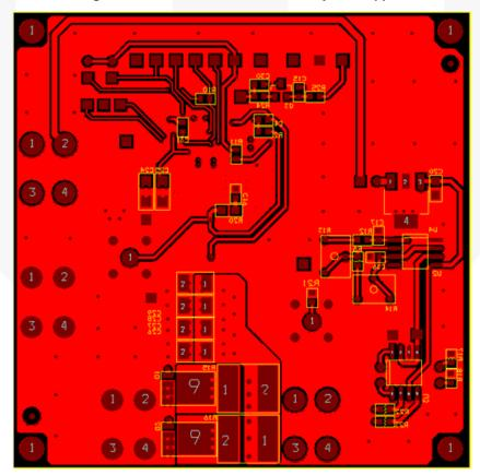
Figure 27. Evaluation Board Bottom Layer Copper
