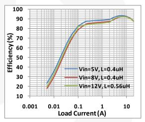
Figure 8. Efficiency vs. Load Current with  $V_{OUT}$ =1.2 V and  $f_{SW}$ =500 kHz
