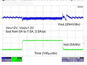
Figure 19. Transition from CCM to DCM Operation
