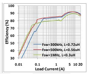
Figure 6. Efficiency vs. Load Current with  $V_{IN}=12\ V$  and  $V_{OUT}=1.2\ V$
