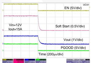
Figure 13. Startup Waveforms with 15 A
