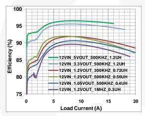
Figure 7. Efficiency vs. Load Current with V<sub>IN</sub>=12 V
