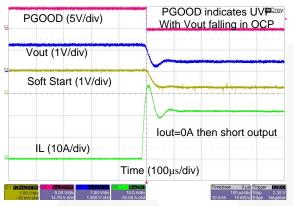
Figure 22. Over-Current Protection with Heavy Load Applied
