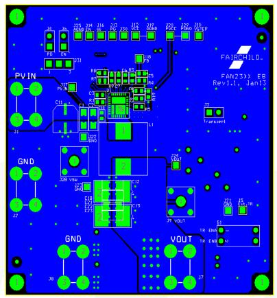
Figure 24. Evaluation Board Top Layer Copper
