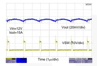
Figure 17. Static Load Ripple at Full Load
