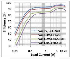
Figure 5. Efficiency vs. Load Current with  $V_{\text{IN}}$ =12 V and  $f_{\text{SW}}$ =500 kHz
