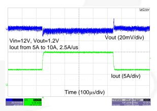
Figure 20. Load Transient from 0% to 50% Load Current
