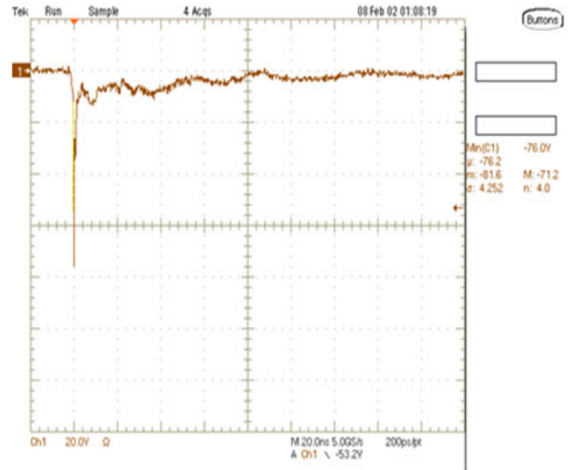
Figure 2. ESD Clamping Voltage Screenshot Negative 8 kV Contact per IEC61000-4-2
