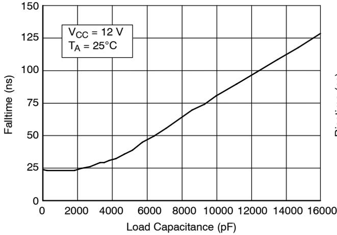
Figure 3. GATE(H) and GATE(L) Falltime vs. Load Capacitance
