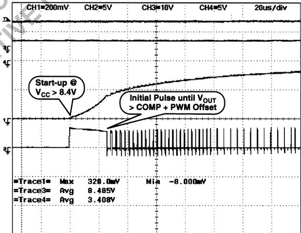
**Figure 10. Normal Startup Showing Initial Pulse Followed by Soft Start (20 μs/div)**
