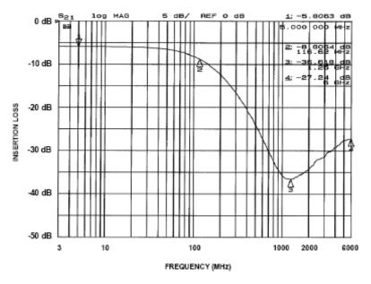
Figure 7. Insertion Loss vs. Frequency (FILTER7 Input to GND)
