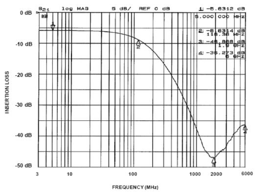
Figure 5. Insertion Loss vs. Frequency (FILTER5 Input to GND)
