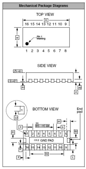
Dimensions for 16-Lead, 0.4mm pitch NuDFN Package
