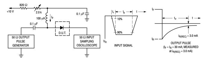
Notes: 1. A 2.0  $k\Omega$  variable resistor adjusted for a Forward Current (IF) of 30 mA.
