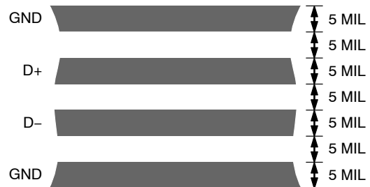
Figure 34. Typical Arrangement of Signal Tracks
