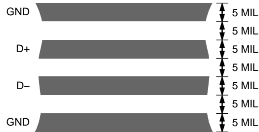
Figure 34. Typical Arrangement of Signal Tracks
