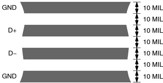
Figure 19. Arrangement of Signal Tracks
