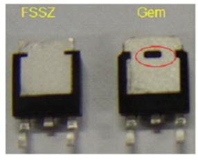
Note: there is a slot hole on GEM heat sink surface for both DPAK and IPAK compared with Fairchild Suzhou (FSSZ) product. There is no impact to the application
