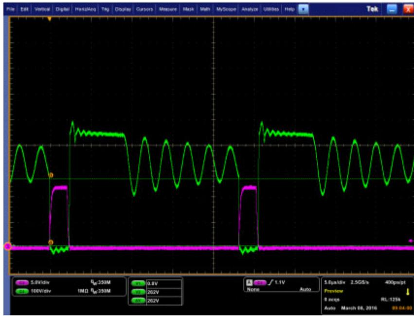
**Figure 7. Valley Switching at 6<sup>th</sup> Valley for Improved Efficiency (Green: Drain voltage, Purple: Drive)**
