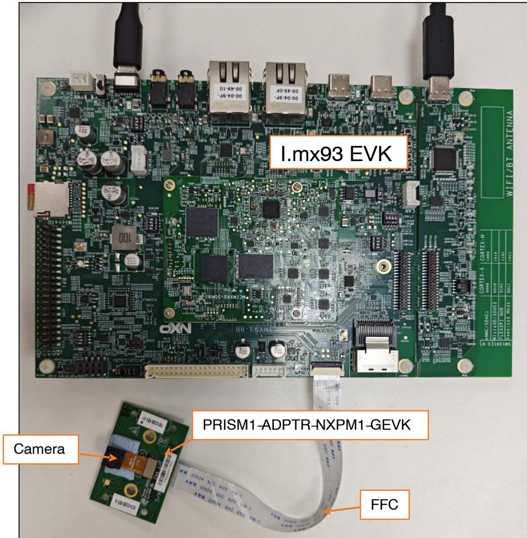
Figure 8. PRISM Module to NXP i.mx93 EVK
