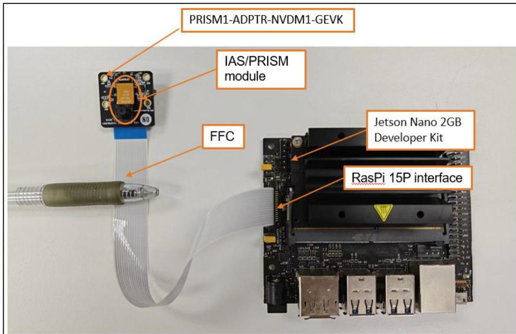
Figure 9. PRISM Module to NVIDIA Jetson Nano EVK
