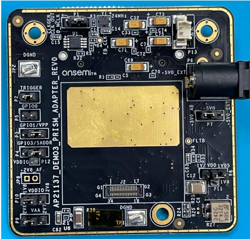
Figure 3. Top Side View of PRISM DEMO3 Adapter
