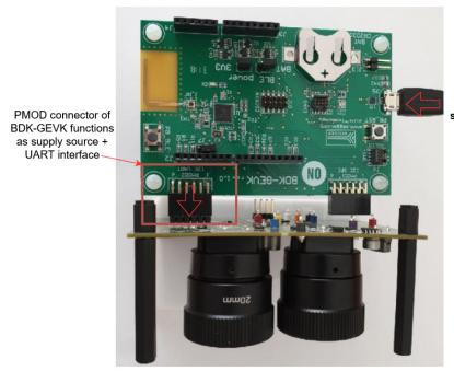
USB - Cable connected to BDK-GEVK.Rangefinder is supplied over PMOD by 3.3.V
