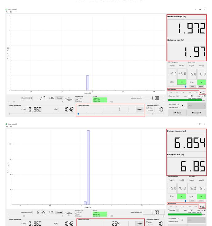
Figure 17. Trigger Pulse Count can be Adjusted between 1-254 Pulses
