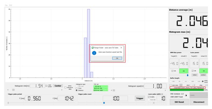
Figure 23. AutoSaving of Measured Data in Trigger Mode for Custom ToF File Name and Storage Destination (Part 3/3)
