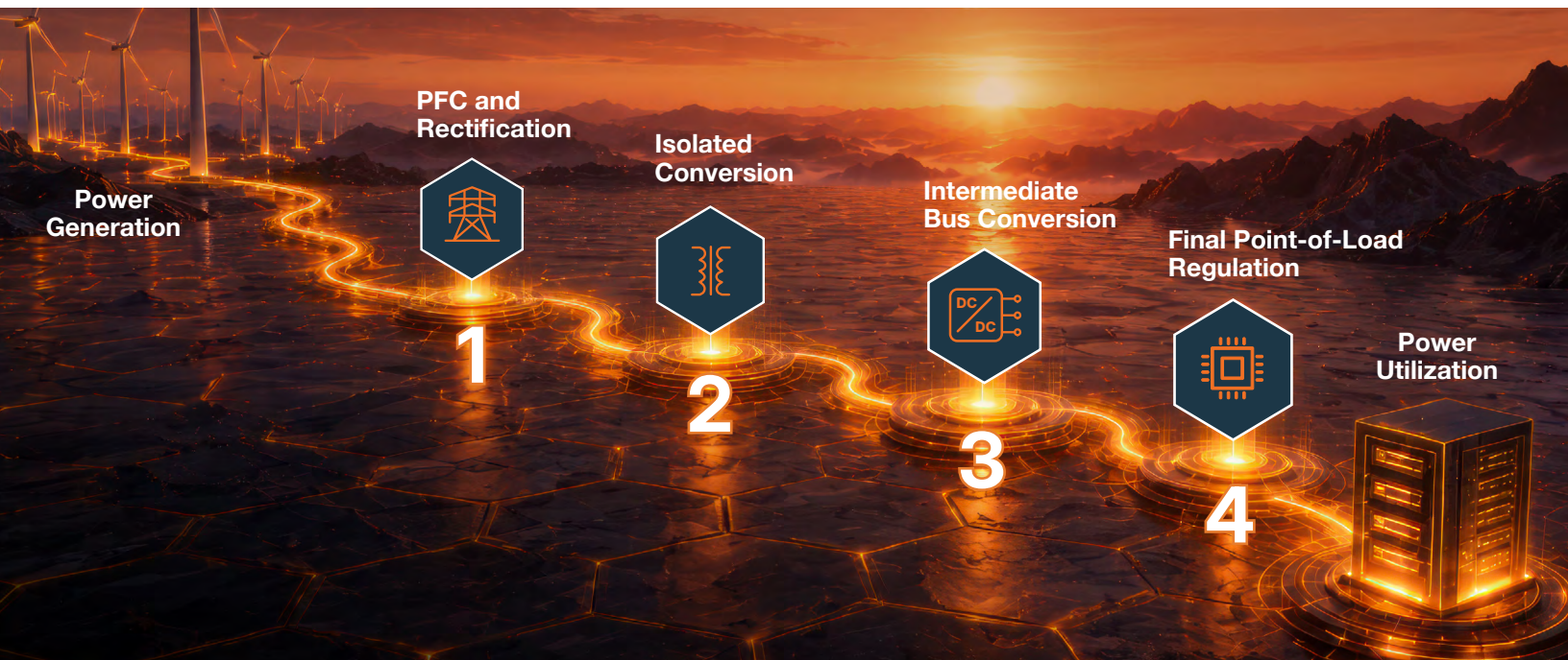
Figure 2. A visualization of the four stages of power conversion, as power flows from its source of generation to its final point-of-load.
