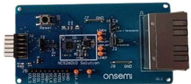
Fig.10: 10BASE-T1S MACPHY Development kit demonstrates the basic functionality and allows to develop software
