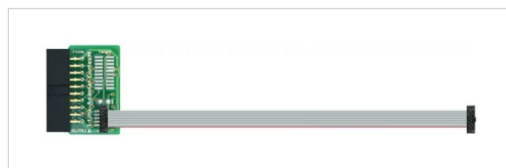
9-Pin Cortex-M Adapter with cable
