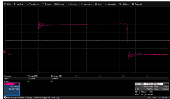
Figure 12. Switching Node (Q3 MOSFET) – Load Step Response @ Input: 12 V, Output Load: 18 V, 1.5 A
