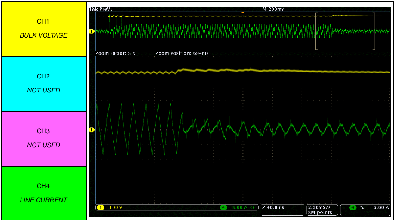
Figure 79. PFC Step Load 1000 W – 200 W @ 230 V AC
