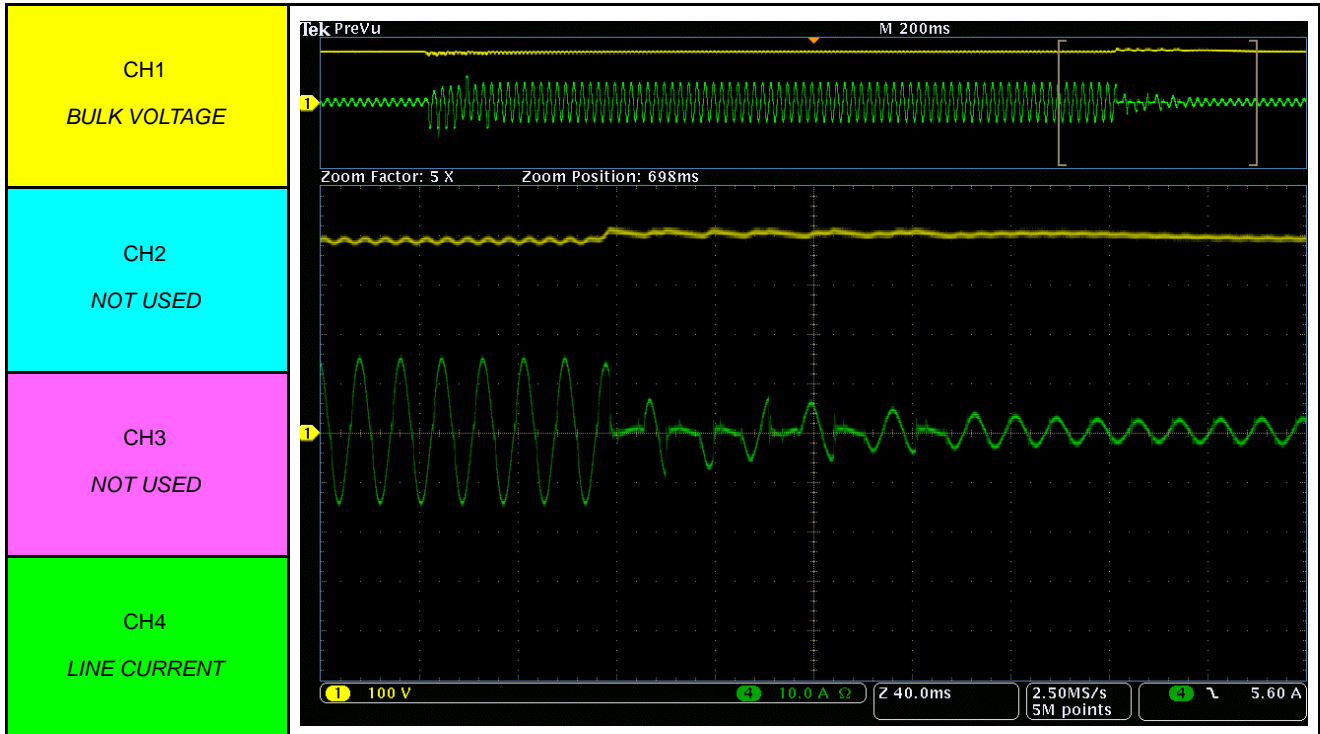
Figure 78. PFC Step Load 1000 W – 200 W @ 110 V AC
