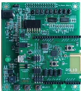
Figure 2. Top Side of the Control Board with the EVBUM2529/D Plug-in
