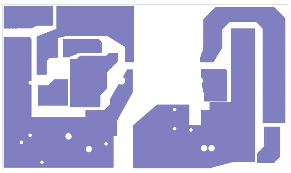
Figure 10. Layout Inner Layer 2
