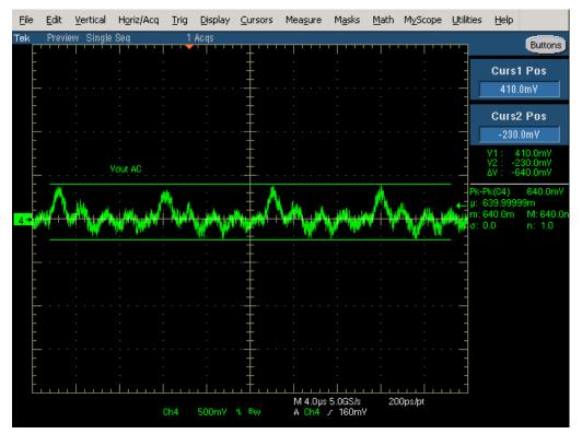
Figure 16. 48 Vin Output Ripple
