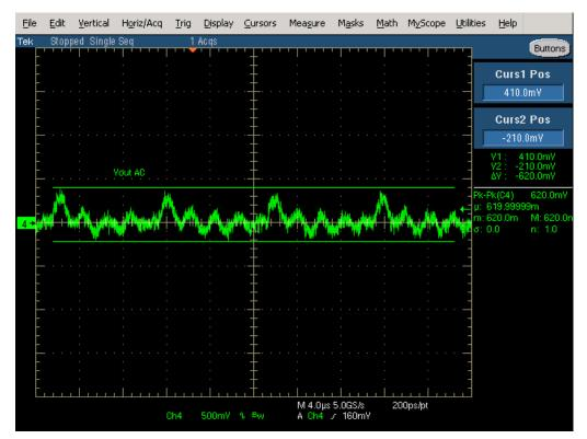
Figure 17. 57 Vin Output Ripple
