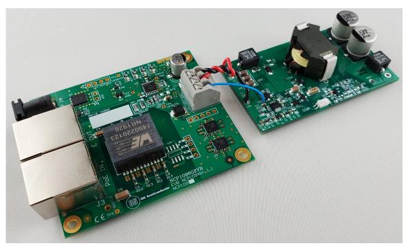
Figure 4. Power over Ethernet Complete Solution with NCP1096GEVB
