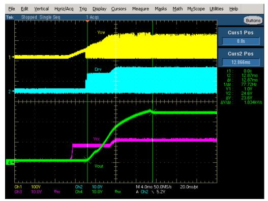
Figure 14. Full Load 48 Vin Startup Waveform
