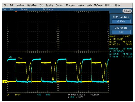
Figure 13. Normal Operating Waveform 48 Vin, 24 Vout, 1.9 A
