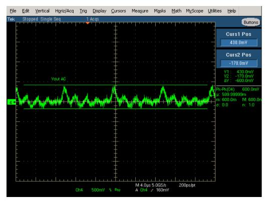
Figure 15. 37 Vin Output Ripple
