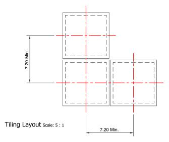
NOTE: Alignment and placement tolerances depend on the accuracy of the equipment used in the assembly process.
